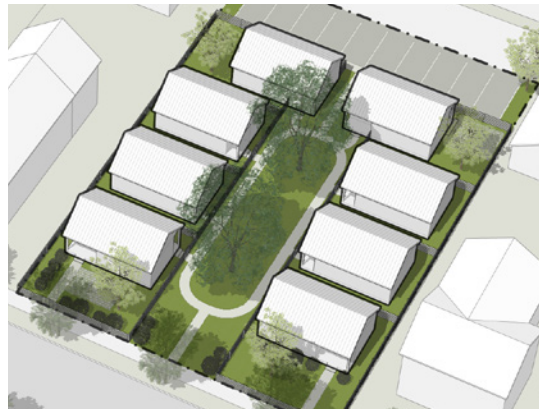
Cottage courts trade smaller lots for shared open space. In the case shown above, two conventional single-family lots are reconfigured to accommodate 7 more affordable “tiny” homes that front a shared common space.
